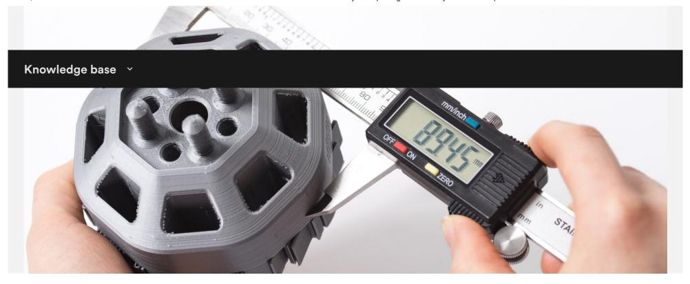
Dimensional accuracy in <u>3D printing</u> refers to how closely the measurements in your <u>CAD design</u> match those of the part once it's printed. It's a key consideration if your components need to fit together precisely or if you're manufacturing sizable assemblies.
